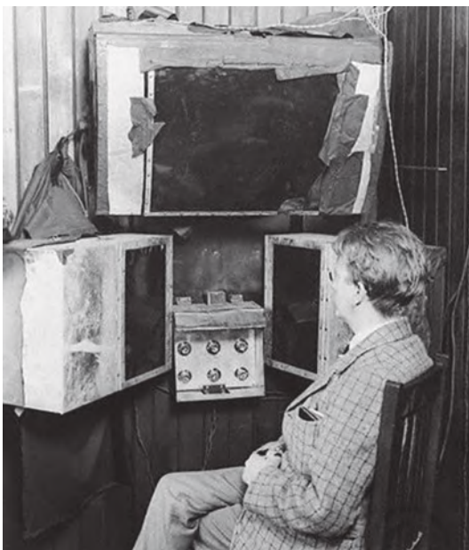
John L. Baird sits in front of the apparatus with which he demonstrated to the Royal Institute, his invention, the 'televisor', an early television.
